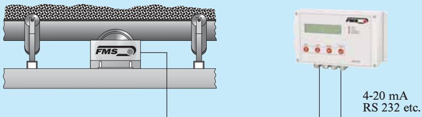
Universal electronic unit for the measurement of daily and total throughput, actual flowrate and belt speed. Various interfaces, such as RS232, analogue outputs, pulse outputs for connection of printer, remote counter or analogue meter. Ready for installation in cabinets or wall-mounting.
