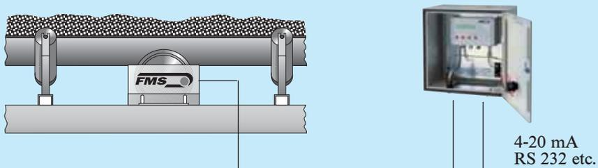
This version of the BMGZ 600 is especially suitable for tough working conditions in mobile units such as crushers and screening units. The electronic unit is available as a single or double channel version. As an option, a fitting frame with rubber buffers can be supplied.
