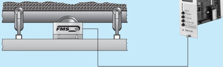
This electronic unit offers all relevant functions in an «OEM version» and was specially designed for installation in 19" systems usually communicating with a PC or an PLC. Complete remote control of the belt weigher is possible via a master system.
